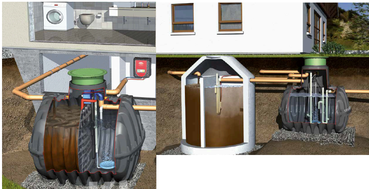
Figure 4-17: Underground tank system for individual house (left) and combination with existing septic tank (right) (GRAF 2017-2)
